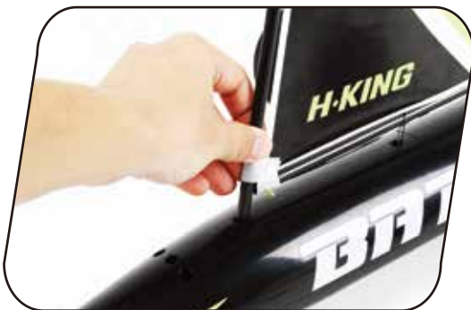
16. Slide the mast into the step block until it bottoms out. The mast should be angled backwards slightly.
