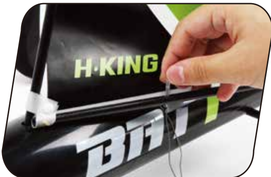
17. Slide 1/2" main sheet tube with line through opening of the boom.
