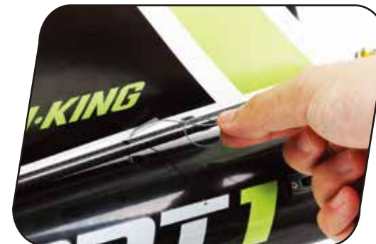
19. Mark end of main sheet line where it exits 1/2" tube.
