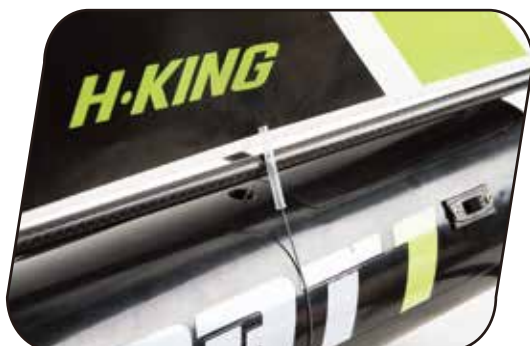
18. Turn On transmitter and receiver. Pulling the trigger all the way, slide 1/2" tube as tight as possible to the boom. Turn receiver Off.
