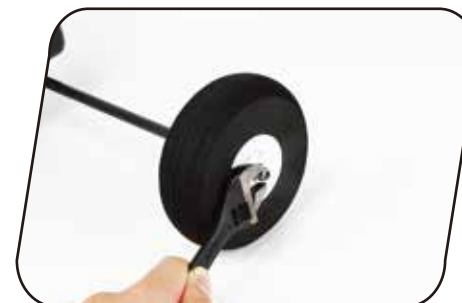
20. Install rear wheels with 8mm nut. Do not over tighten bearings, wheels should spin freely.
