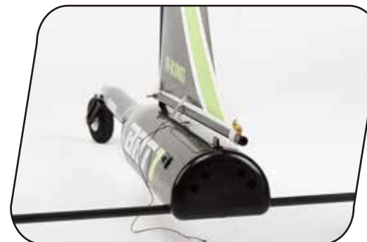
19. With the transmitter on, push the trigger all the way forward, giving you excess slack in the main sheet line. Tie a double knot at the location you marked on the main sheet line. Test control setup by pulling the trigger all the way back again. The main sheet line should be taught, allowing little side to side movement of the boom.
