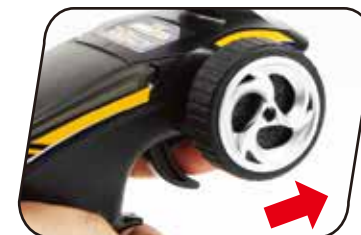
19. With the transmitter on, push the trigger all the way forward, giving you excess slack in the main sheet line. Tie a double knot at the location you marked on the main sheet line. Test control setup by pulling the trigger all the way back again. The main sheet line should be taught, allowing little side to side movement of the boom.
